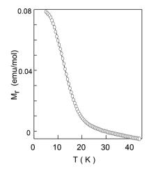
Fig. 12 Remanent magnetization as a function of the temperature for  $Sr_2CoTeO_6$ .
