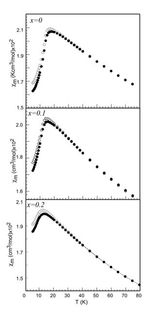
Fig. 11 FC and ZFC magnetic susceptibility curves in the  $Sr_2Co_{1-x}-Mg_xTeO_6$  ( $x=0.0,\,0.1,\,0.2$ ) series.
